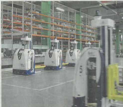
Les robots sans fil et autonomes de BA Robotic Systems Group effectuent le transport de charges. Photo BA Robotic Systems
